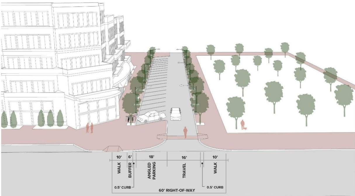
Figure 18.47.8, Typical Cross Section for Millcreek Common Street
