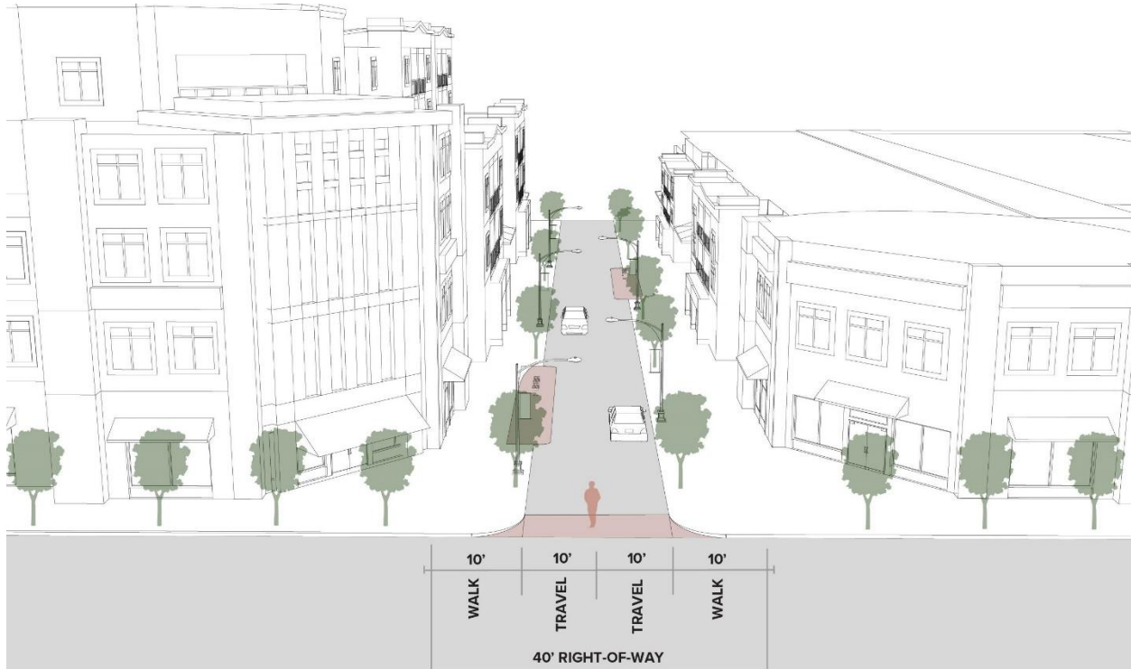
Figure 18.47102, Typical Cross Section for Woonerf
