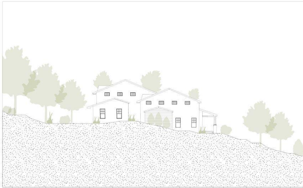
Figure 18.61.2, A Development Plan that Minimizes Cuts
